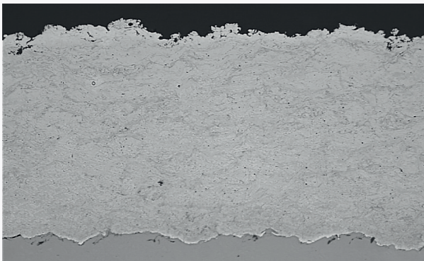
HVOF Cu Coating 275 \mu\text{m} Thick, Porosity <0.5%
