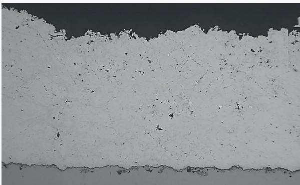
HVOF Al Coating 225 \mu\text{m} Thick, Porosity <1%
