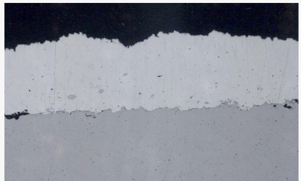
HVOF Ag coating 200 \mu\text{m} thick, porosity <0.5%
