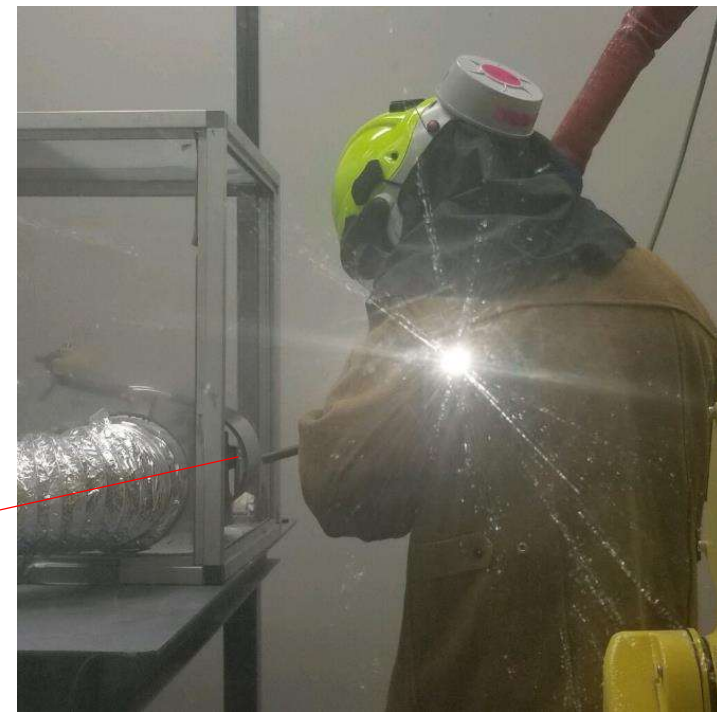
Manual Cold Spray operation using 410SS based repair material
