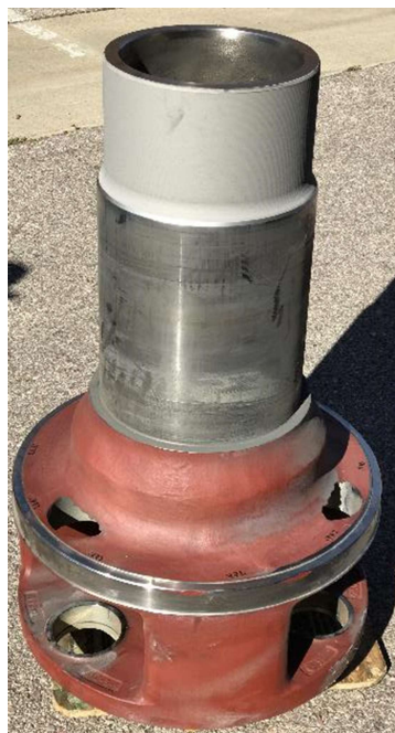
After cold spray repair
