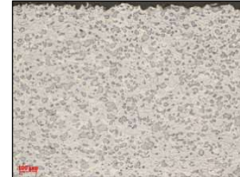
High density barrier coatings of nickel or stainless steel
