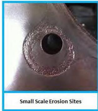
Cylinder Head – Flat Erosion Sites away from Fire Surface
